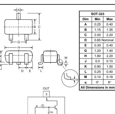
IN GND(0) Schematic and Pin Configuration
